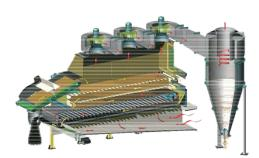
The system consists of individual cyclones with the extractor fans mounted on a common hood. Each fan is provided with Dampers to set the air balance. 'Portholes' are provided for easy cleaning & inspection.
